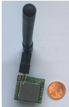
Fig. 1: LoRa transceiver inAIR9b: Semtech's chip sx1276, 868-915 MHz [2].
