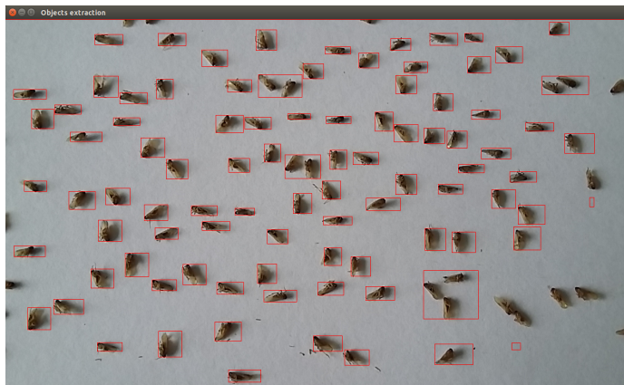
Figure 2: Brown Planthopper counting (93/106 individuals - accuracy 88%). The image is taken at 1280x720 resolution with around 50cm distance. In average, each individual has 52.08x30.67 pixels shape and contributes roughly 1063.7 pixels in the image.
